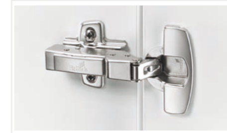
Name Hettich 110° hinge with integrated silent system Code PWWM0016 Notes Applied to half-overlay doors and door thickness ≤ 22mm
