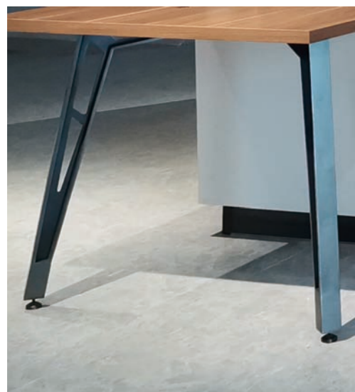
Name F-shaped Double Support Legs Code PWNB0038 Size -H870mm, adjustable height range: 0-20mm -Material: stainless steel, grey color, two legs per set (pads and metal legs included). And the distance between the legs can be adjusted according to the bartop size.
